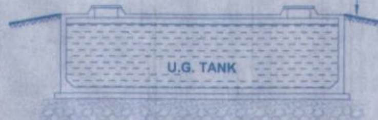
TYPICAL SECTION THRU. U.G. TANK SCALE: NTS
